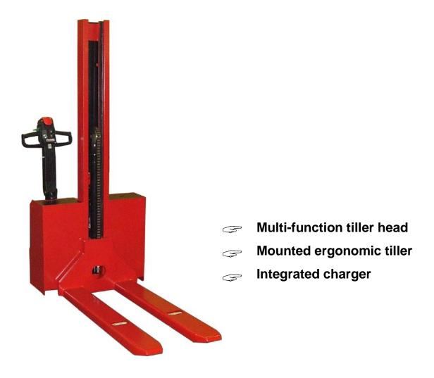
The Electric truck - pedestrian stacker compact ERV - 10 combines performance efficiency and operator friendliness in one attractive design. It provides a multitude of utilisation possibilities for practically any application. For example: depositing goods on racking or feeding machines. Palletised goods are simply lifted to the required picking height and are then deposited in the racking without stressing the back or taken from the pallet.
