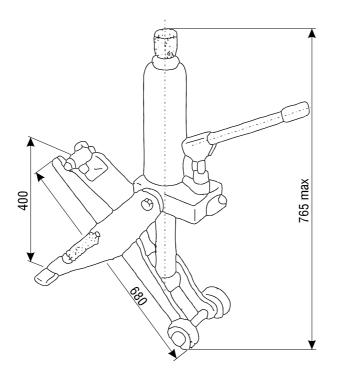
Load capacity - 8 t Maximum lifting weight - 400 mm
